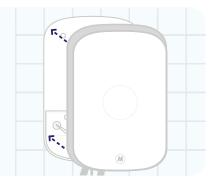
14. Attach the sensors to the water heater pipes.
